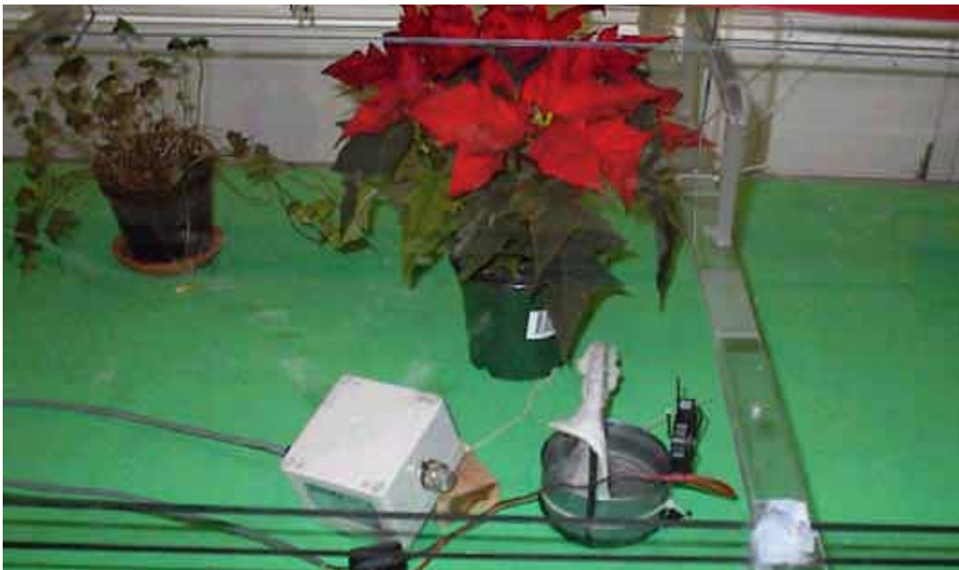
Figure 7. Omega HX93 Relative humidity and temperature sensor (Omega Engineering Inc 2003)
